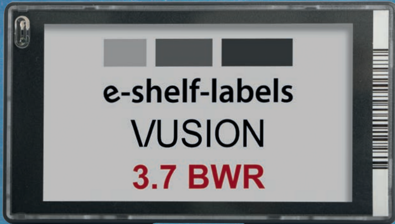
Display: 81,54 x 47,04 mm optional Easylock, Displayschutz, LED
