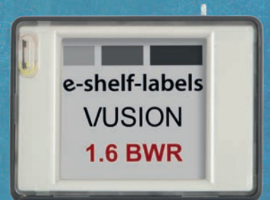
Display: 27,5 x 27,5 mm optional Easylock, Displayschutz, LED
